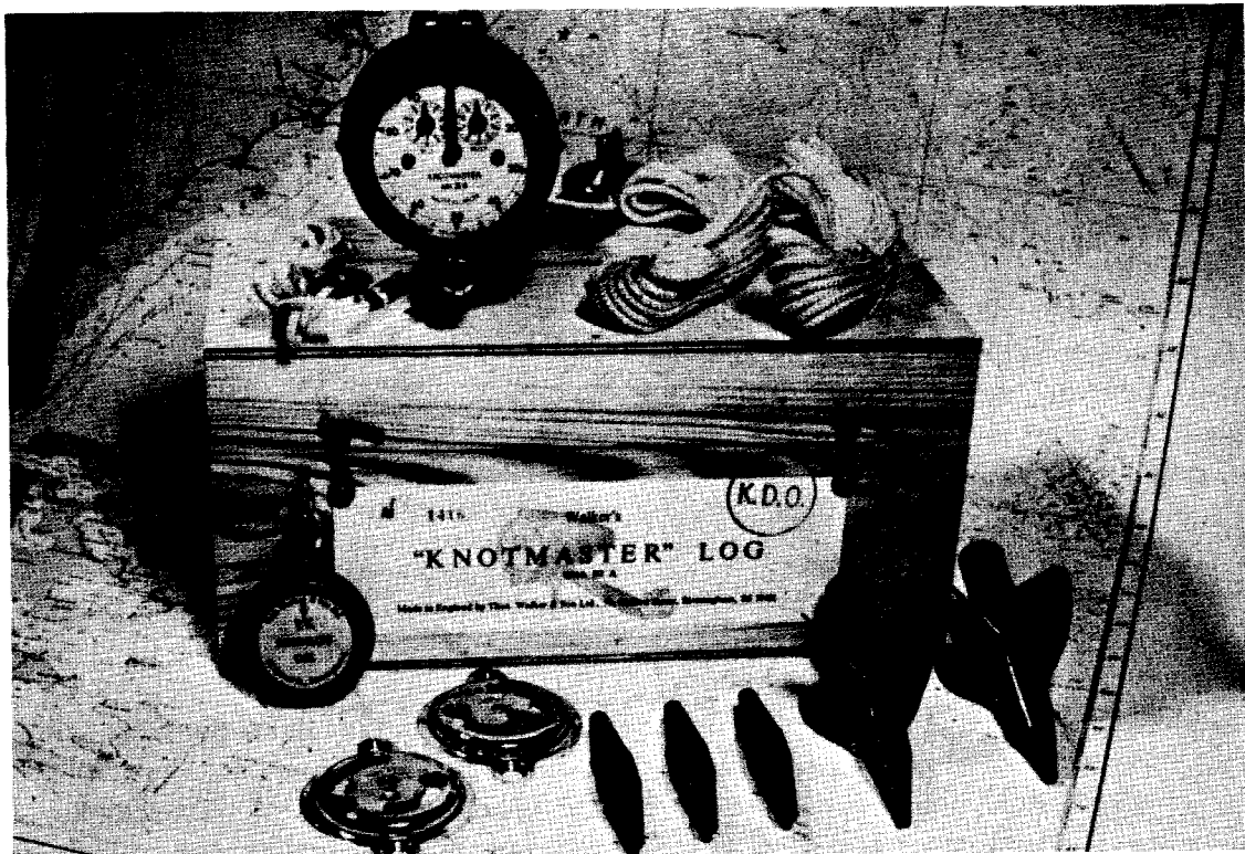
A reliable distance log, like this Walker KDO Knotmaster Log for boats up to 40 feet, helps the offshore navigator maintain an accurate dead-reckoning position. Courtesy Weems & Plath, Inc.
